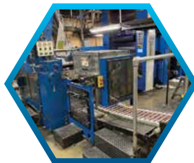
The machine folds the newspapers and is belt delivered.
