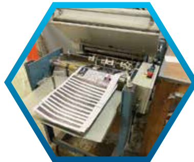
In the folding process press sheets are untouched until they are stacked and handled by staff wearing gloves on the edge of the paper.
