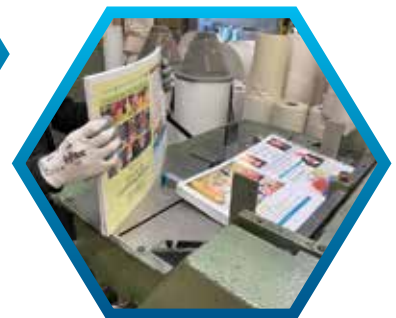
In the binding process gloves are worn to reduce touching of the products and the edges are trimmed off in the process reducing to near-zero human touch.
