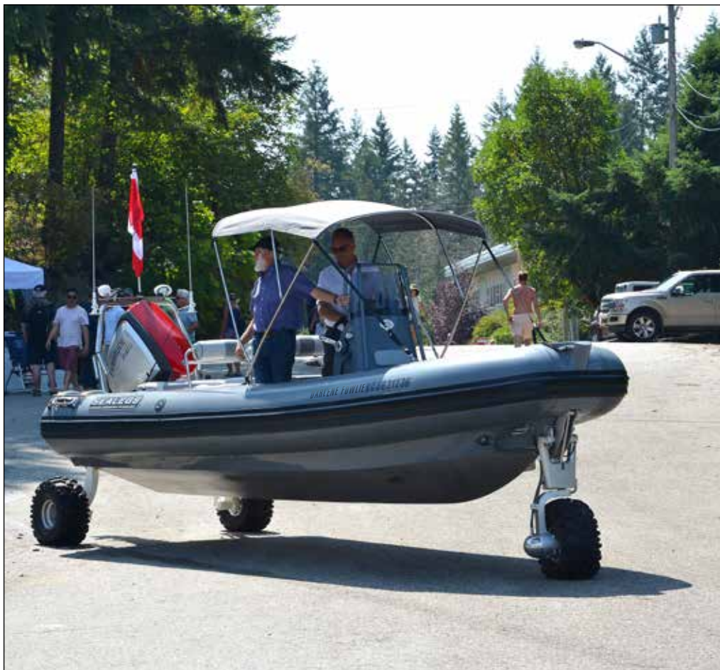
How long will it be before one of these are seen driving through Madeira Park? Sea Legs offered Pender Harbour Days attendees demonstrations of their amphibious boats. The system consists of motorized, retractable and steerable wheels fitted to specially designed boats 'to give users a fully integrated, turn-key package.'
