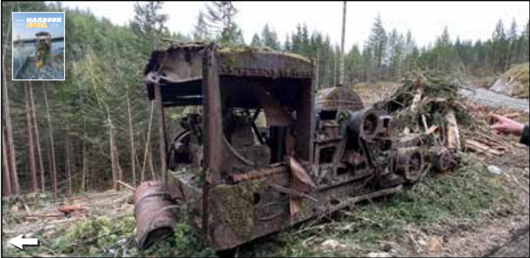
APRIL: Recent logging in Egmont has uncovered this gas-powered yarder from the 1940s or 1950s.
