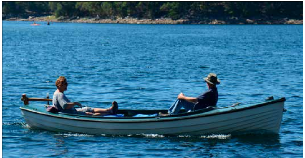
Ursula and Doug Hardwick aboard their own Pender Harbour Launch design, a 16-foot fibreglass clinker-style cruiser. You won't hear them coming because the boat is powered by a 24 volt, 3/4 horsepower electric motor that gets her up to 5 knots.
