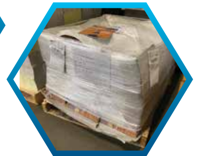
Finished product is stacked on a skid and protective shrink wrap is used to secure the product before delivery.
