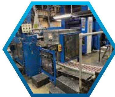
The machine folds the newspapers and is belt delivered.
