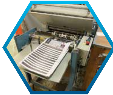
In the folding process press sheets are untouched until they are stacked and handled by staff wearing gloves on the edge of the paper.
