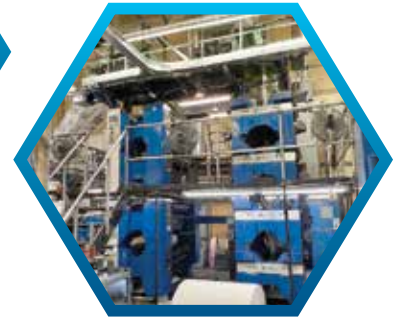
The paper is pulled untouched through the machine at 30,000 copies per hour.
